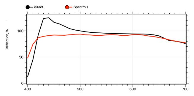
does not have any ultraviolet to activate the fluorescent standard. The measurement confirms this, since the expected blue fluorescence peak is absent from the resulting spectrum. Thus the Spectro 1 is always using an M2 measurement condition.
