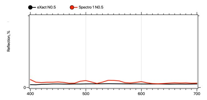
The higher Spectro 1 reflectance differences are below 1%, possibly due to specular reflection, sensor drift, dark noise or all of them.
