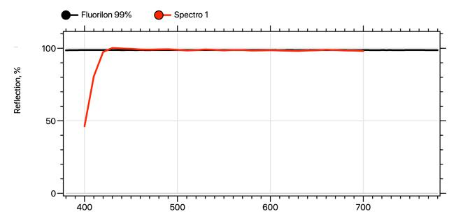
The results are good from 420 to 700 nm, but below from 400 to 420 nm the instrument is displaying dramatically reduced response.
