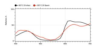
As expected, the Spectro 1's white LED does not have any UV light emission to excite the fluorescent inks, so the high fluorescent peaks were reduced. However, the instrument did not refuse to measure any of the inks. Amazingly it did try its best to give a spectrum within its range that would produce a color similar to the inks.
